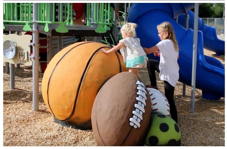
A fun sports themed climber with varying degrees of climbing difficulties. Constructed of durable Glass Fiber Reinforced Concrete (GFRC). The unique design allows for 360 degrees of climbing, integrated handholds, realistic texture.
