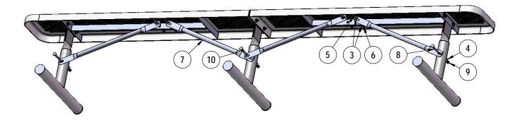
Attach the 26-3/4" Braces to the Seats and Legs as shown using specified hardware.
