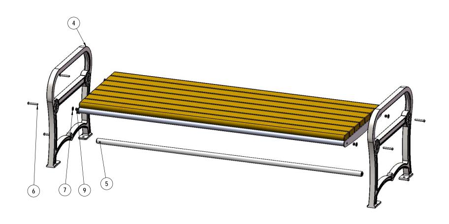
Attach the 6' Seat Frame and Support Bar to the Cast End Frames using the specified hardware.
