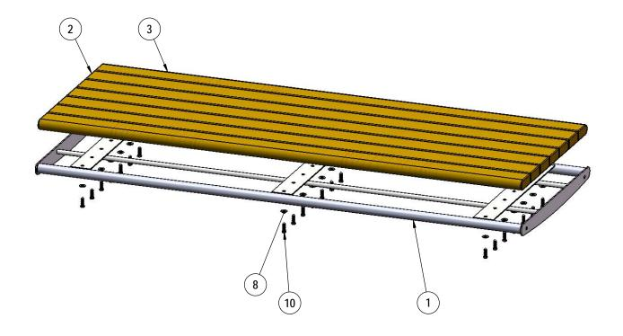
Attach the 6' Recycled Planks to the Seat Frame using the specified hardware.
