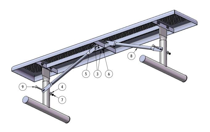
Attach the 26-3/4" Braces to the Legs using specified hardware as shown.
