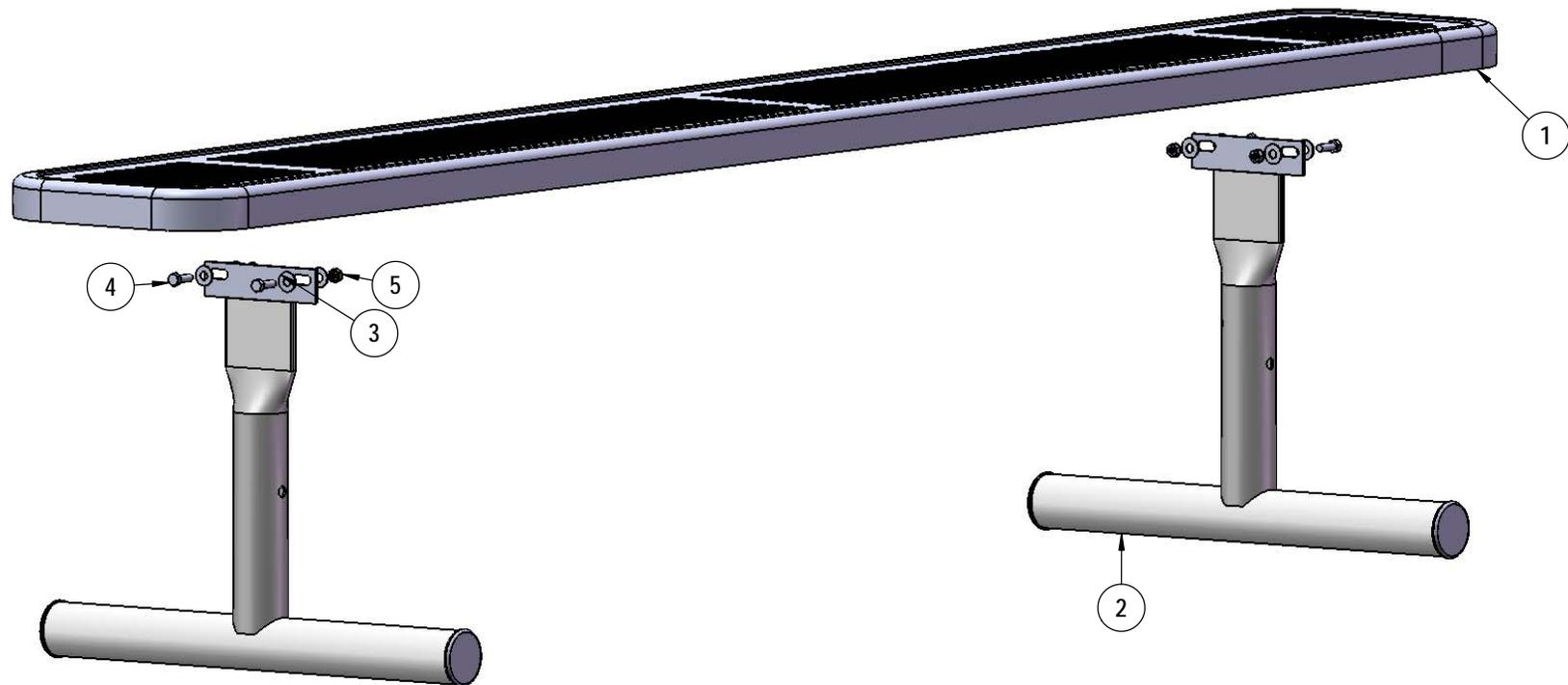
Attach the 8' Punched Seat to the Legs using specified hardware.
