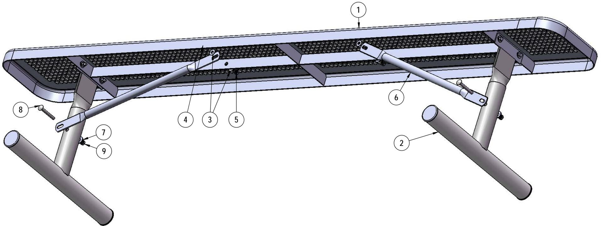
Attach the 26-3/4" Braces to the 8' Seat and Legs using specified hardware as shown.
