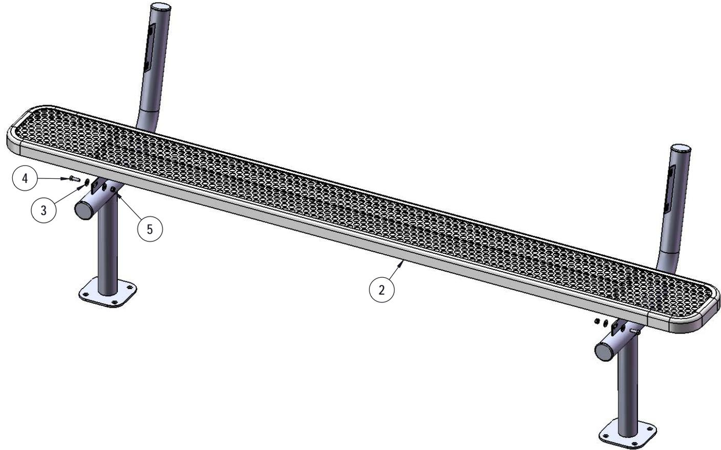
Attach the seat plank to the Legs using specified hardware.
