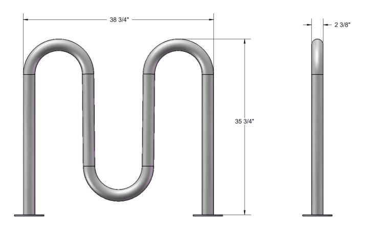
Recommended Surface Mount Hardware: 3/8" x 3-1/2" Concrete Expansion Anchor Bolts
