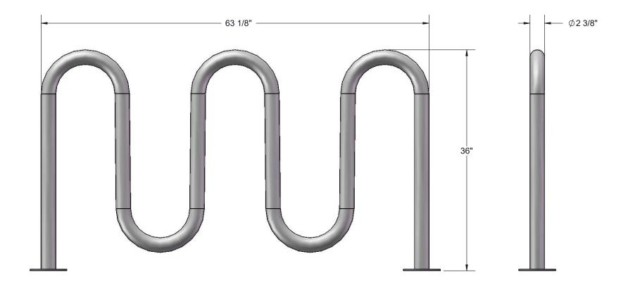
Recommended Surface Mount Hardware: 3/8" x 3-1/2" Concrete Expansion Anchor Bolts
