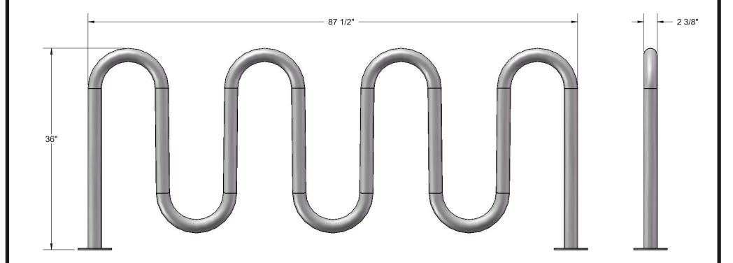
Recommended Surface Mount Hardware: 3/8" x 3-1/2" Concrete Expansion Anchor Bolts
