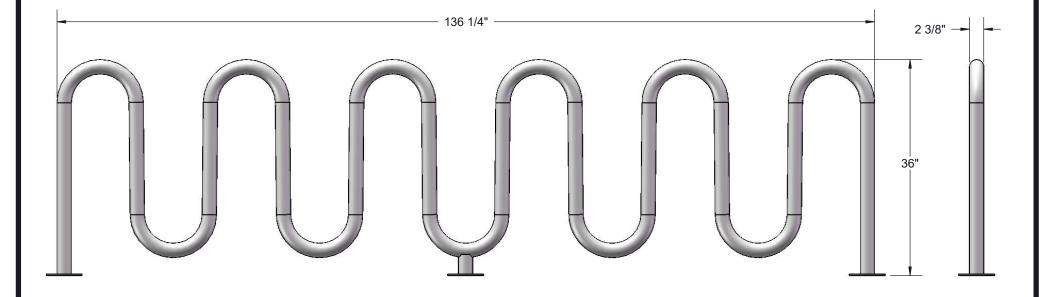
Recommended Surface Mount Hardware: 3/8" x 3-1/2" Concrete Expansion Anchor Bolts
