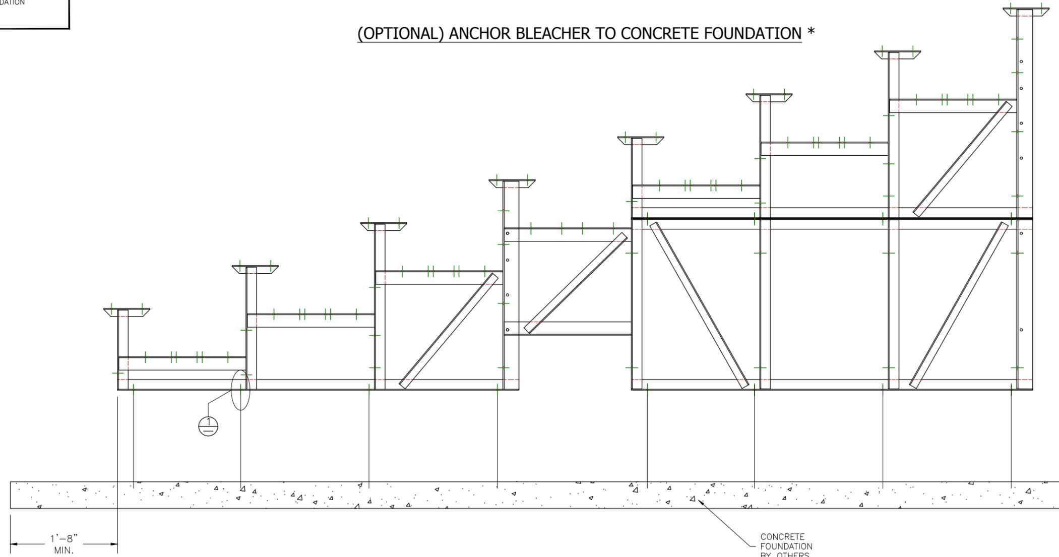
\* CONCRETE WEDGE ANCHORS NOT INCLUDED WITH ALL UNITS. IF USING OTHER ANCHORING SYSTEM, SKIP THIS STEP AND REFER TO INSTRUCTIONS SPECIFIC TO THE ANCHORING SYSTEM PURCHASED FOR YOUR UNIT. SEE PRINT FP.1 (INCLUDED IN THIS PACKET) FOR GENERAL CONCRETE FOUNDATION SPECIFICATIONS.
