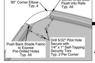
Downward Mounting Plate Points Straight Downward Pre-Drilled Holes in Typ. All Rail Ends Face Inward to Center of Frame 1-1/4" x 70-13/16" Typ. All Frame End Rail Typ. 2 1-1/4" Curved Side Rail with Mounting Plate Typ. 2
