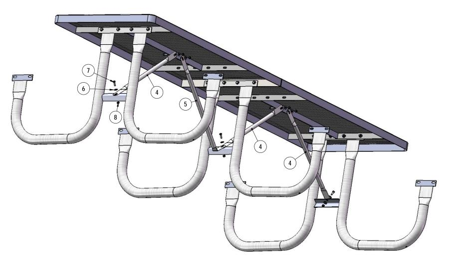
Attach the braces to the frame and under side of the top as shown using specified hardware.
