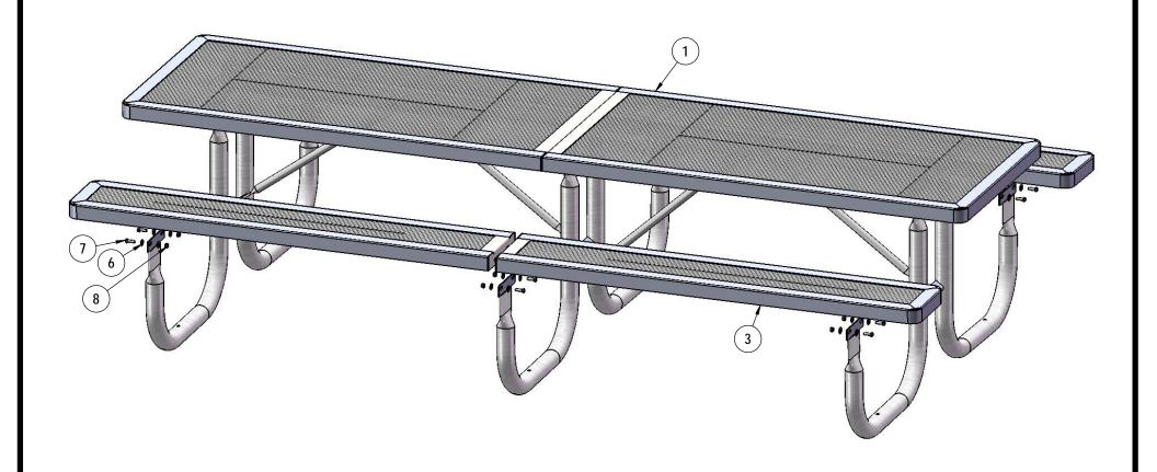
Attach the seats to the frame as shown using specified hardware.
