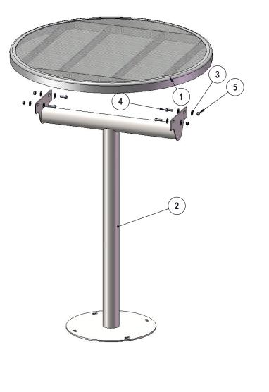
Required surface mount hardware: 3/8" x 3" concrete expansion anchor bolts (not included)
