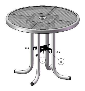
Attach the Spreader Plate to the leg assembly as shown using specified hardware.
