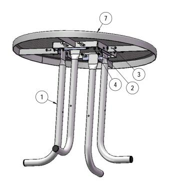
Attach the 36" Top to the Legs as shown using specified hardware.
