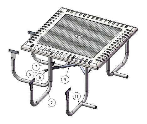
Attach the Cross Brace to the 358 Legs using specified hardware.
