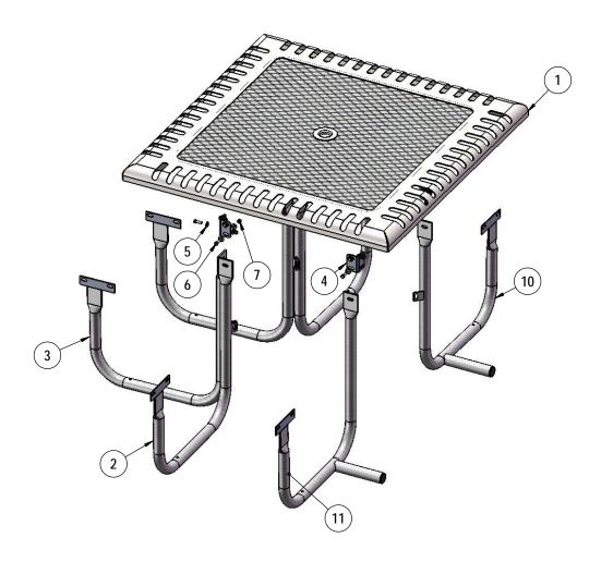
Attach the 358 Legs to the 358 Top using the specified hardware.
