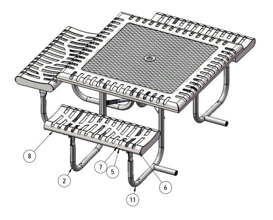
Attach the seats to the legs as shown using specified hardware.
