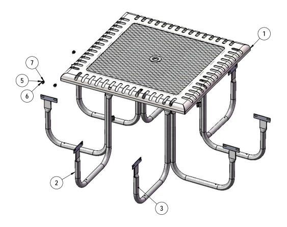
Attach the 358 Legs to the 358 Top using the specified hardware.
