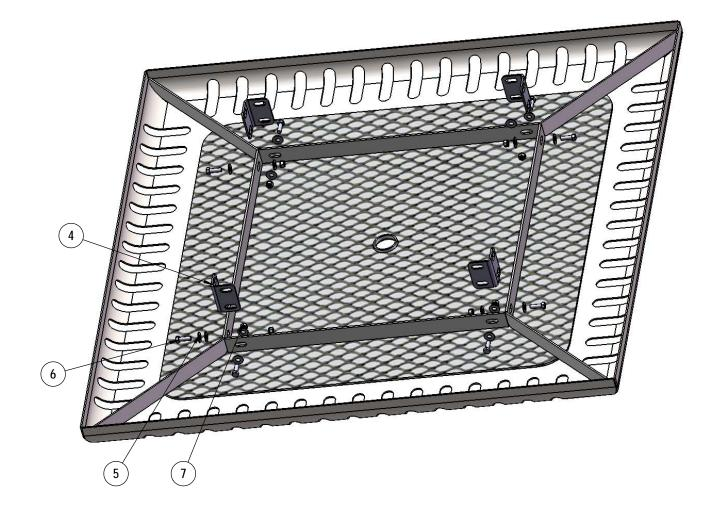
Attach the 358 Extension Tabs to the 358 Top using the specified hardware.
