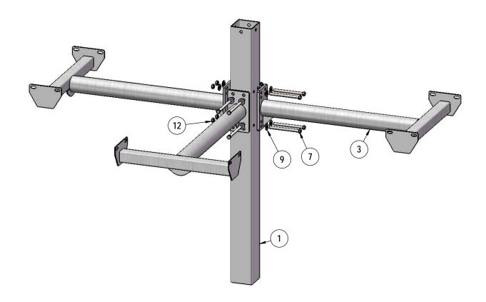
Attach the seat arms to the post as shown using specified hardware.
