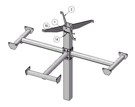
Attach the H Bracket to the post as shown using specified hardware.
