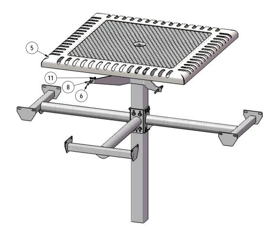
Attach the top to the H Bracket as shown using specified hardware.
