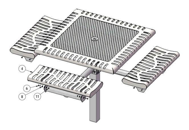
Attach the seats to the seat arms as shown using specified hardware.
