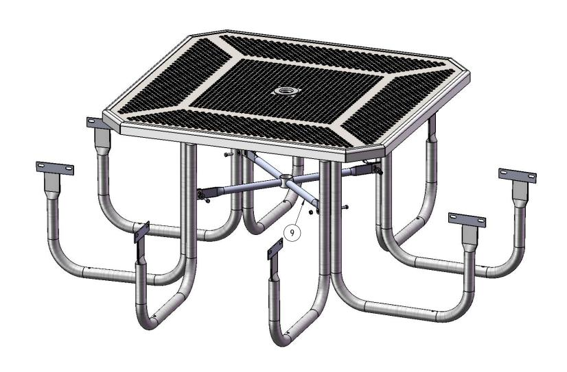
Attach the Crossbrace between the table legs as shown using specified hardware.
