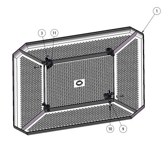
Attach the Extension Tabs to the Top using specified hardware.
