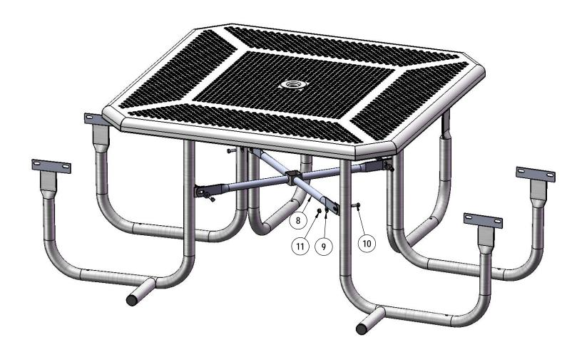
Attach the Crossbrace between the table legs as shown using specified hardware.
