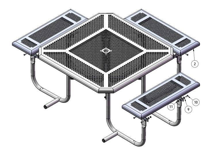
Attach the 3' Seats to the Legs using specified hardware.
