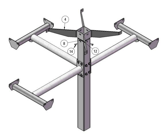
Attach the H Bracket to the Post using specified hardware.
