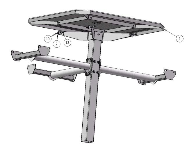
Attach the 46" Octagon Top to the H Bracket using specified hardware.
