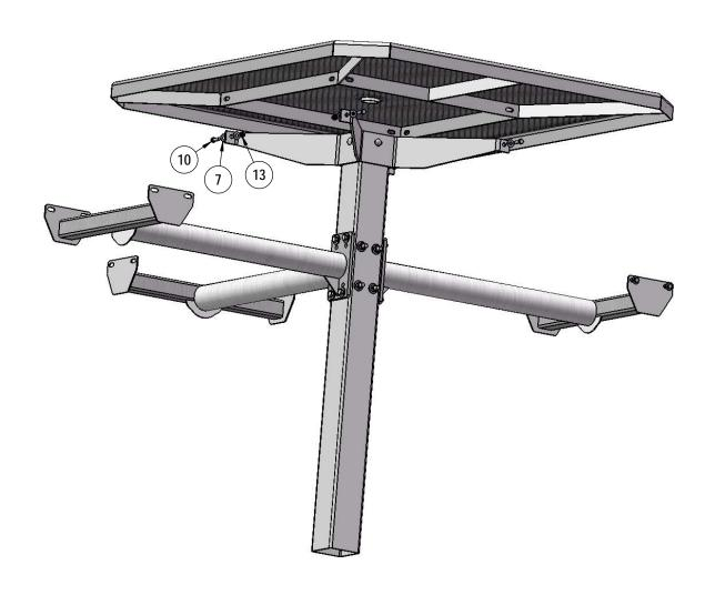
Attach the 46" Octagon Top to the H Bracket using specified hardware.
