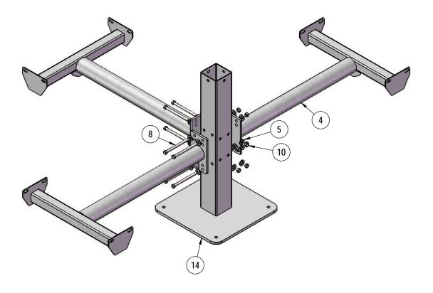
Attach the Arms to the Post using specified hardware.
