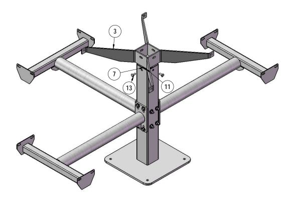
Attach the H Bracket to the Post using specified hardware.
