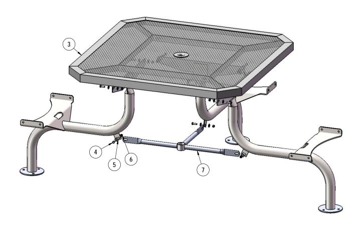
Attach the legs to the top as shown using specified hardware. Then attach the cross brace to the legs.
