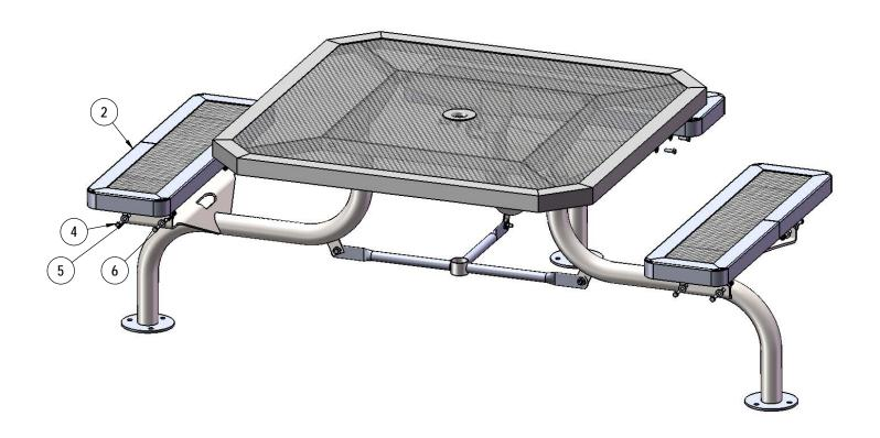
Attach the seats to the legs as shown using specified hardware.
