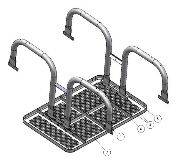
Attach the Frames to the 4' Punched Top using the specified hardware.
