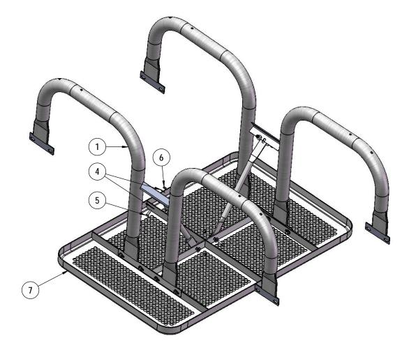
Attach the 21-3/8" Braces to the 4' Punched Top and the Frames as shown using specified hardware.
