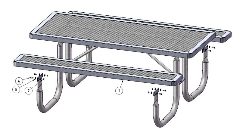
Attach the seats to the frame as shown using specified hardware.
