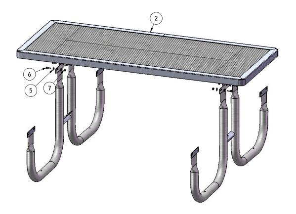
Attach the top to the top legs as shown using specified hardware.
