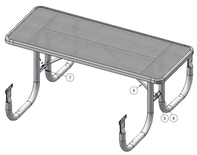
Attach the 29 7/8" braces to the Legs using specified hardware.
