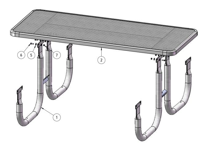
Attach the 6' Top to the Legs using specified hardware.
