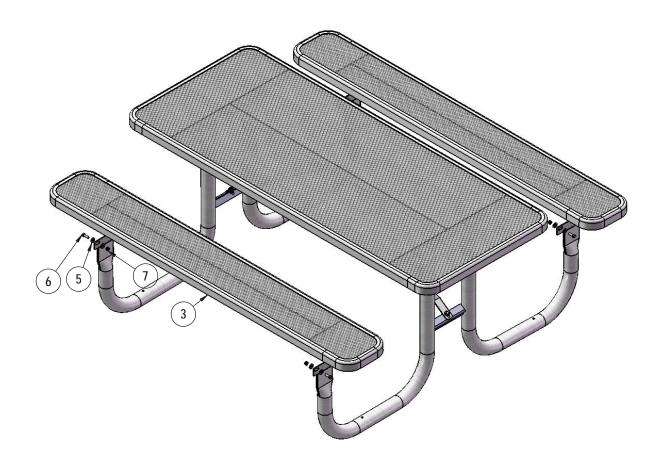
Attach the 6' Seats to the Legs using specified hardware.
