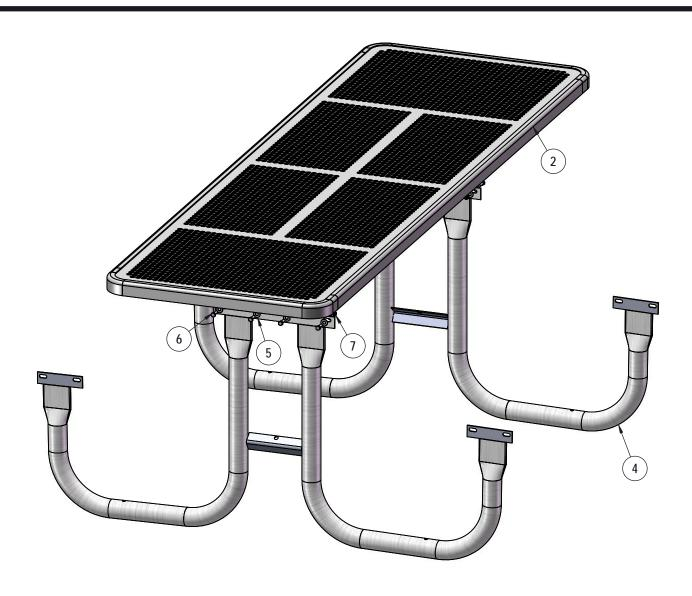
Attach the 8' Handicap Punched Top to the Frames using specified hardware.
