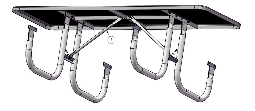
Attach the 29-7/8" Braces to the 8' Handicap Punched Top and the Frames as shown using specified hardware.
