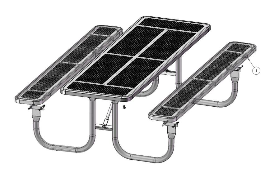
Attach the 6' Punched Seats to the Frames using specified hardware.
