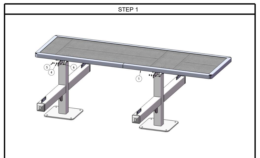
Attach the top to the post assemblies as shown using specified hardware.
