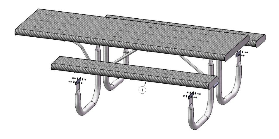
Attach the 6' Vinyl Rolled Seats to the Frames using specified hardware.
