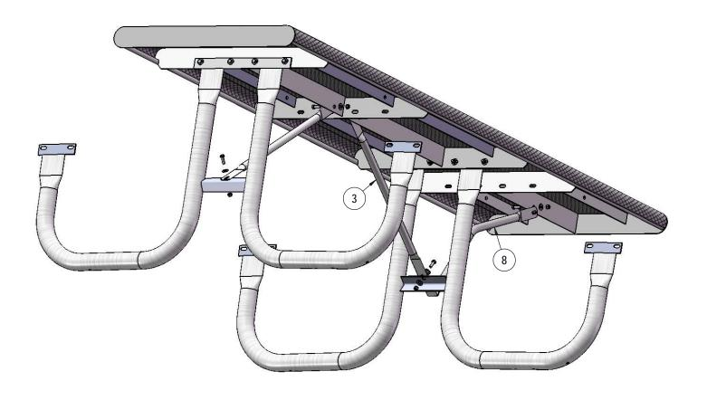
Attach the 29-7/8" Braces to the 8' Vinyl Rolled Top and the Frames as shown using specified hardware.
