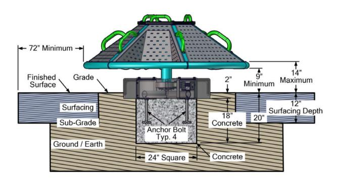
Shield Mounting Brackets Must Be Level Typ. All Center Shaft Must Be Plumb **Bracket Sets on Concrete** Typ. All
