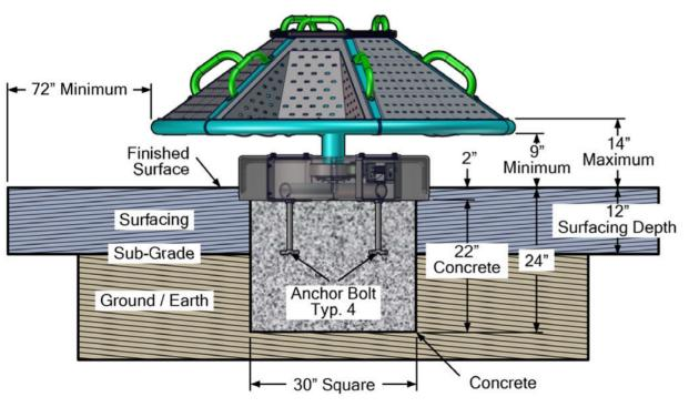
Concrete Forms and Framing Provided by Installer Allow Concrete to Cure Based Upon Manufacturer's Specifications. Recommended Cure Time is **7 Days**. Concrete Required: 11.5 ft³ - 0.42 cubic yards
