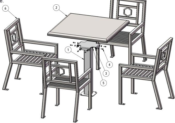
Recommended Surface Mount Hardware: 3/8" x 3" Concrete Expansion Anchor Bolts (Not Included)
