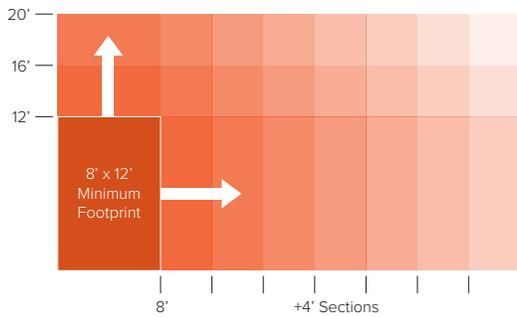
The Cycle Station 2 can be sized to meet your capacity needs. Starting with a width of 12', 16' or 20', you can add on as many 4' lengths as needed.
