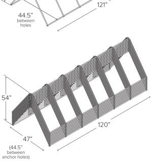
14 Bikes CAPACITY **MATERIALS** .75" steel tube **FINISHES** Galvanized An after fabrication hot dipped galvanized finish is our standard option. **MOUNT** Surface only **OPTIONS**
