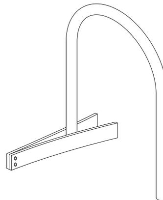
An easy way to brace the rack while the grout sets is to bolt two 1x4" boards together at one end and clamp them onto the legs of the rack like a clothes pin.
