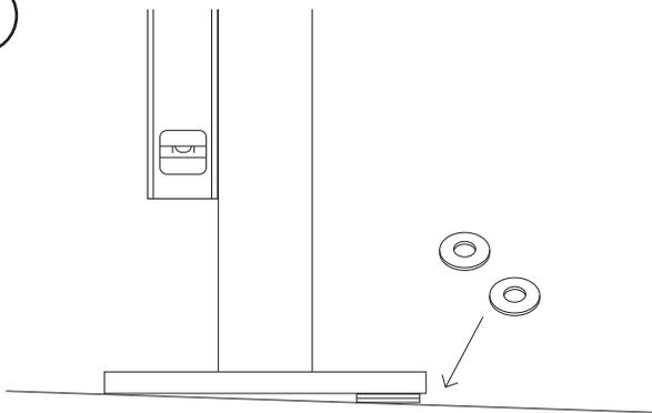
Place rack (and washers to level rack if necessary) over holes.
