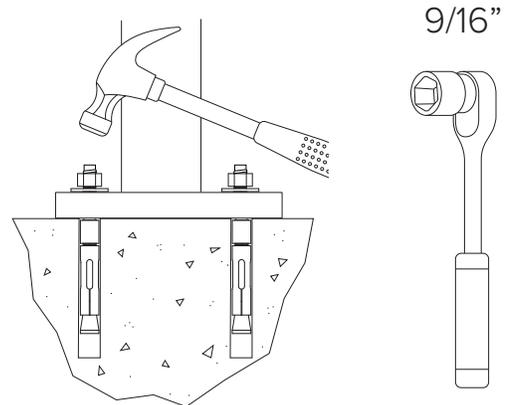
Thread nuts onto anchors, leaving approximately 1/4" of the anchor protruding, and tap into surface. Tighten nuts down to secure rack.
