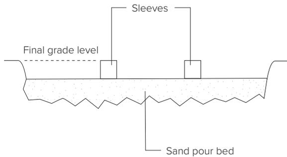
Place corrosion resistant sleeve (min. 3" inside diameter) in sand pour bed in exact location where rack will be installed. Make sure top of sleeve is at same level as desired finished concrete surface. Fill sleeve with sand to keep it in place and prevent it from filling with concrete.
