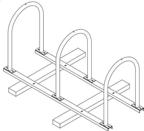
Place racks on beams so holes in rack flanges line up with beam slots
