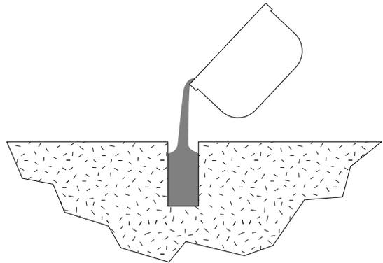
Fill holes with Super Por-Rok or epoxy grout.
