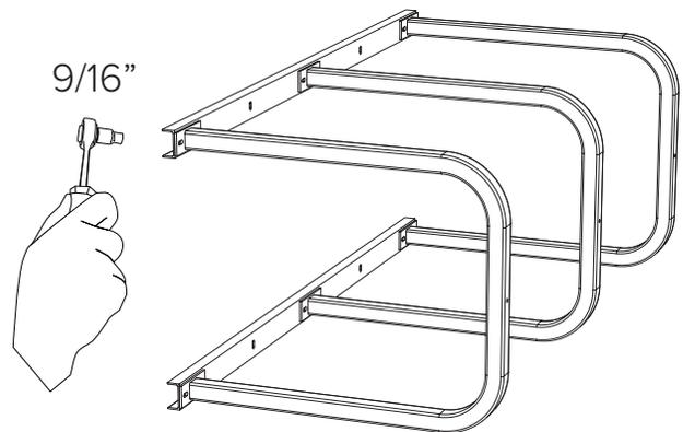
Once nuts are on, tip assembled rack over and use a 9/16" socket to tighten nuts. Before fully tightening nuts, make sure the racks are straight on beams. If using tamper resistant nuts, use access tool to tighten nuts. Do not overtighten the tamper resistant nuts. Tip rack upright.
