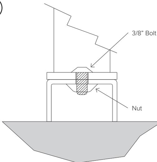
Put bolts through rack flange holes and beams so bolt head faces up. **HAND** tighten the nuts using new flange nuts.
