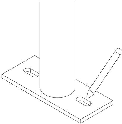
Place the rack in the desired location. Use a marker or pencil to outline the holes of the flange onto the base material.
