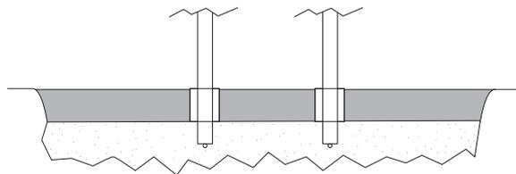
After appropriate cure time, dig out sand from sleeves and insert rack, making sure it is level and at the appropriate height. Pour in Super Por-Rok or epoxy grout and allow to set.
