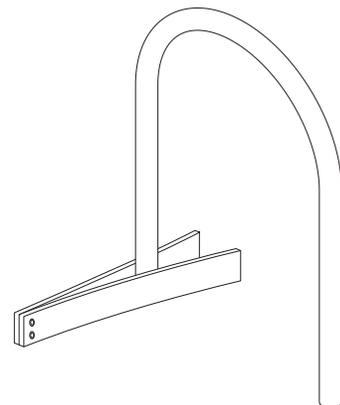
An easy way to brace the rack while the grout sets is to bolt two 1x4" boards together at one end and clamp them onto the legs of the rack like a clothes pin.
