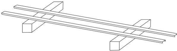
Lay out the two channel beams where the rack will be placed. Place the two beams on top of the two blocks of wood so that the open part of the channel faces the ground.
