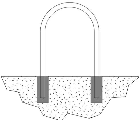
Place rack into holes, making sure it is level until the grout has set. 33"-36" of the rack should remain above the surface.
