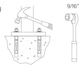
Thread nuts onto anchors, leaving approximately 1/4" of the anchor protruding, and tap into surface. Tighten nuts down to secure the stand.
