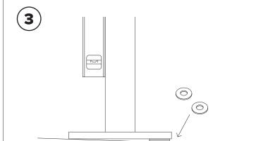
Place Tool Kit (and washers to level rack if necessary) over holes.
