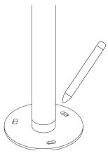
Place the Tool Kit in the desired location. Use a marker or pencil to outline the holes of the flange onto the base material.
